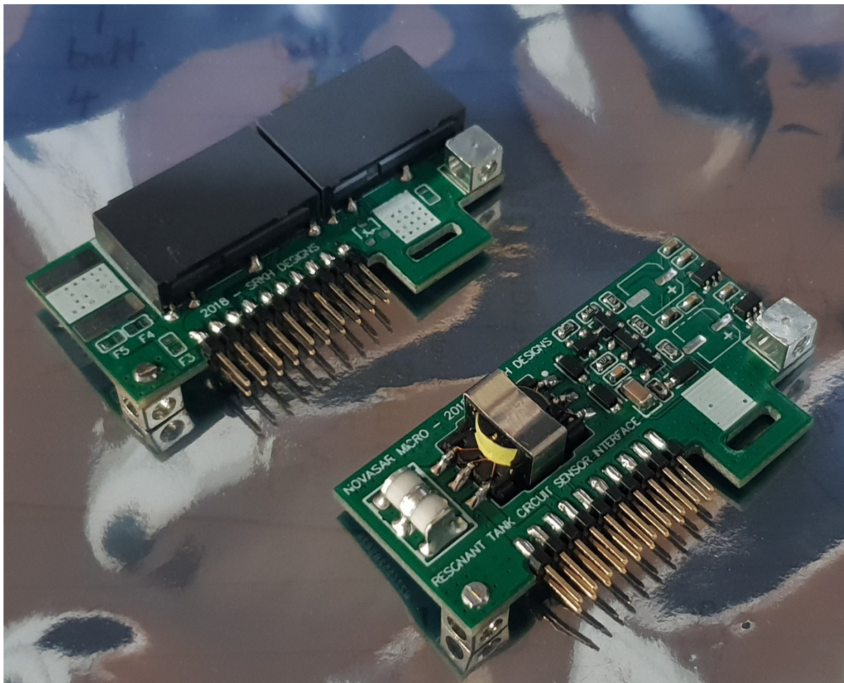
Multi channel relay board (top) and tank circuit inductive loop vehicle detector (bottom).
